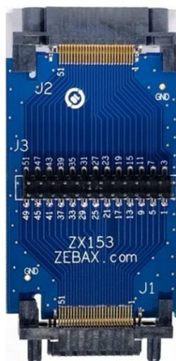
Designed in 4 layers 50Ω trace impedance control. Available GND test point for ease of interface with scope or any test equipment.
