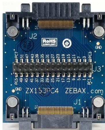
Designed in 4 layers 50Ω trace impedance control. Available GND test point for ease of interface with scope or any general test equipment.
