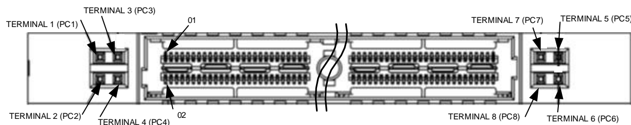
QMS/QFS PC4 terminal ( PC1 .. PC8 ) assignments – front view - 2 bank connector is shown
