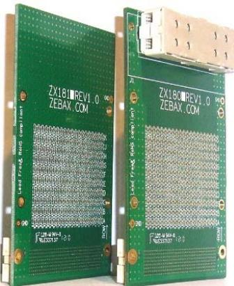
[ZX180FCI](#) and [ZX181FCI](#) daughter cards are introduced supporting FCI MegArray ( Meg-Array) connectors in passive FPGA Mezzanine Card, FMC , breakout adapter application.
